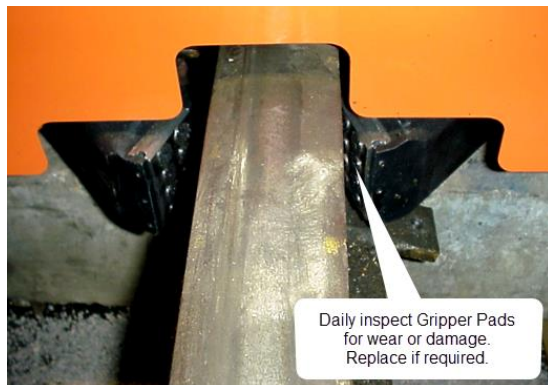
Gripper Cams on Stationary End
