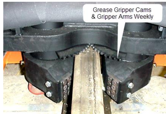
Rail Gripper Cams on Working End
